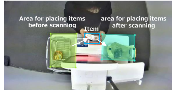
The number of items brought in is estimated by counting the movement of taking out the items from the area for placing items before scanning and putting the items into the area for placing items after scanning.
